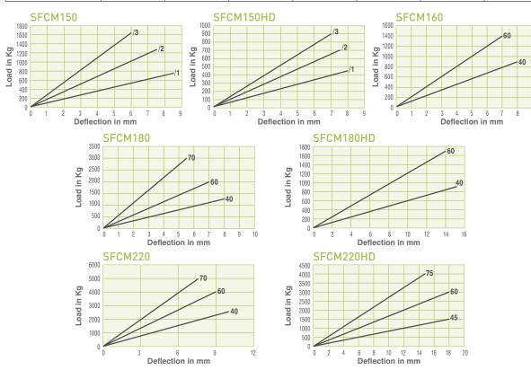
Max compression load in Kg deflection in mm.
