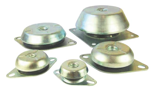
A universal mounting, popular in a wide range of applications. Cost Effective, High Performing and Easy to Install. The rubber is used in shear compression providing optimum performance and offers vibration reduction of up to 95% in all axis. The metal top cap provides protection from contamination such as Oil and Fuel. Load Ratings from 20kg to 5,000kg.
